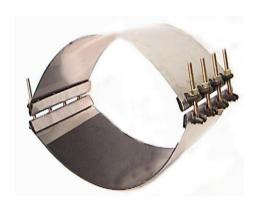
The REMCO 1285EZ Pipe Repair Clamp Series is designed to serve as a quick and economical repair solution for leaks in low pressure applications. Anti corrosive stainless steel band and Zinc Di-Chromate plated fasteners help to ensure long and dependable service. Multi-Panel configuration allows for larger
